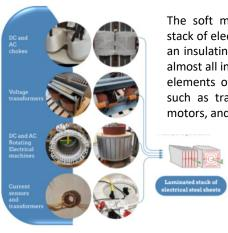
The soft magnetic materials, made from stack of electrical steel sheets separated by an insulating layer, are becoming crucial in almost all industrial sectors, as they are key elements of industrial electrical machines such as transformers, sensors, actuators, motors, and generators.
